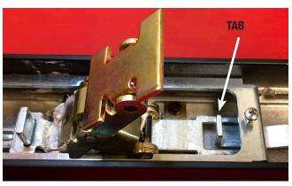
**6.** Once plunger bracket is past tab tighten screw all the way to prevent the bracket from moving forward.
