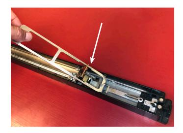
**5.** Make sure the plunger bracket slides all the way to the back where the screw is past the tab.
