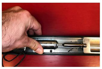
**10.** Move solenoid mount up towards plunger & install remaining (2) screws to mount. DO NOT TIGHTEN!
