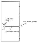
**STEP 2**: Run the wires from the ETH hinge through the 3/8" raceway starting at the ETH hinge & exiting into the pocket.
